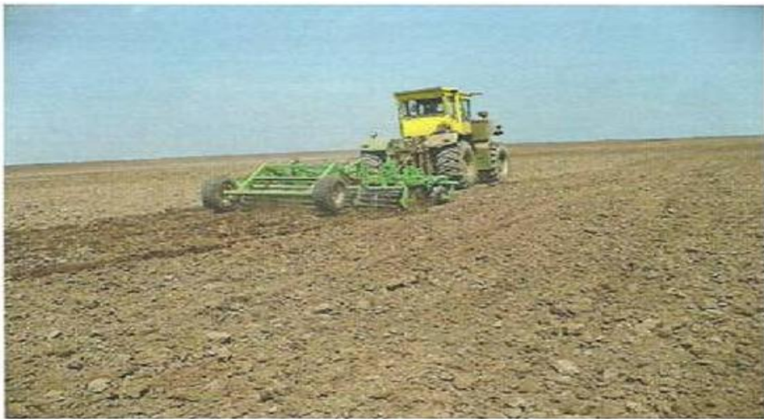
Fig. 1 Aspect during working tests of GD-4 disc harrow
