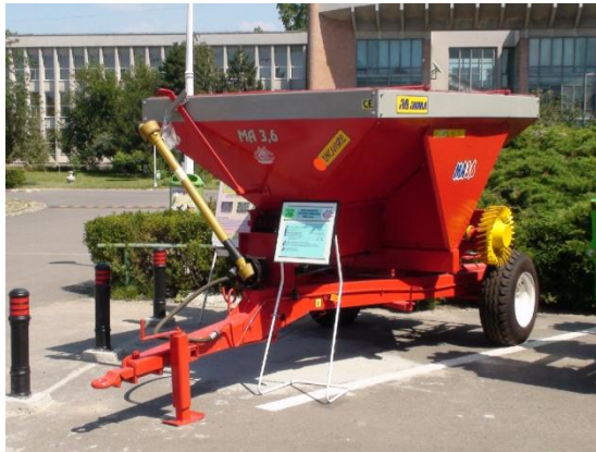
a) b) Fig.1. Machine of applying solid chemical fertilizers, MA 3.6 a) front perspective view b) rear perspective view
