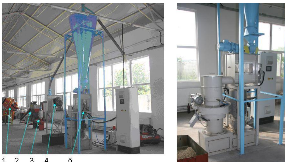
Figure 2. Necessary technical equipment for the pellet agri-pellet production process 1 - agricultural/forestry residue mixer AU; 2 – inclined conveyer belt TIB-0; 3- press feeding transporter TAP-0; 4 – refiner; 5 – pelletizing press.
