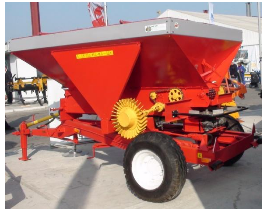
a) b) Fig.1. Machine of applying solid chemical fertilizers, MA 3.6 a) front perspective view b) rear perspective view
