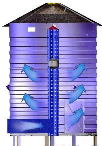
Fig. 3 Aeration through a central column
