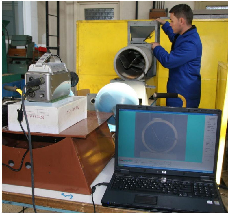
Fig. 5. Stand for investigating the working process of cylindrical sorting machines with alveolis
