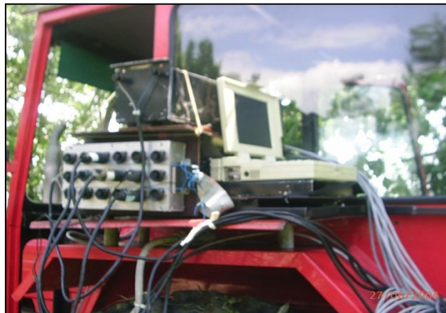
Fig. 4 The data acquiring and interpreting system on the left side of the tractor
